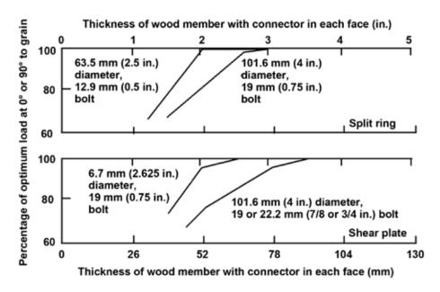
Figure 8–24. Effect of thickness of wood member on the optimum load capacity of a timber connector.
