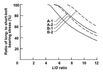
Figure 8–10. Variation in bolt-bearing stress at the proportional limit perpendicular to grain with *L/D* ratio. Relations obtained from experimental evaluation for materials with average compression perpendicular stress of 7,860 kPa (1,140 lb in<sup>-2</sup>) (curve A–1) and 3,930 kPa (570 lb in<sup>-2</sup>) (curve A–2). Curves B–1 and B–2, modified relations used for establishing design loads.
