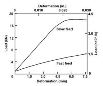
Figure 8–15. Typical load–deformation curves showing the effect of surface condition of bolt holes, resulting from a slow feed rate and a fast feed rate, on the deformation in a joint when subjected to loading under bolts. The surface conditions of the bolt holes were similar to those illustrated in Figure 8–14.
