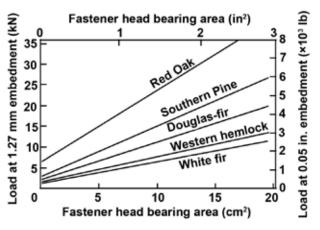
Figure 8–30. Relation between load at 1.27-mm (0.05-in.) embedment and fastener bearing area for several species.
