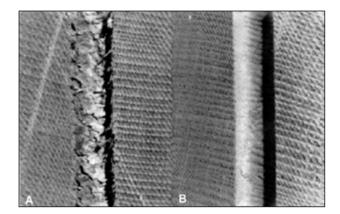
Figure 8–14. Effect of rate of feed and drill speed on the surface condition of bolt holes drilled in Sitka spruce. A, hole was bored with a twist drill rotating at a peripheral speed of 7.62 m min<sup>-1</sup> (300 in min<sup>-1</sup>); feed rate was 1.52 m/min (60 in min<sup>-1</sup>). B, hole was bored with the same drill at a peripheral speed of 31.75 m min<sup>-1</sup> (1,250 in min<sup>-1</sup>); feed rate was 50.8 mm min<sup>-1</sup> (2 in min<sup>-1</sup>).
