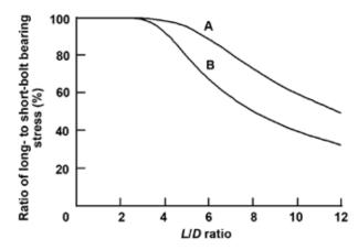
Figure 8–12. Variation in the proportional limit bolt-bearing stress parallel to grain with L/D ratio. Curve A, bolts with yield stress of 861.84 MPa (125,000 lb in<sup>-2</sup>); curve B, bolts with yield stress of 310.26 MPa (45,000 lb in<sup>-2</sup>).
