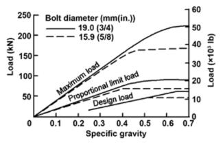
Figure 8–21. Relation between load bearing parallel to grain and specific gravity (ovendry weight, volume at test) for two 101.6-mm (4-in.) shear plates in airdry material with steel side plates. Center member thickness was 88.9 mm (3-1/2 in.).
