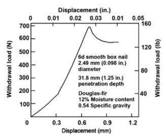
Figure 8–2. Typical load–displacement curve for direct withdrawal of a nail.
