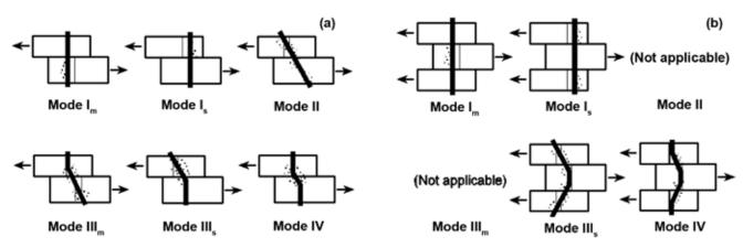
Figure 8–5. Various combinations of wood-bearing and fastener-bending yields for (a) two-member connections and (b) three-member connections.
