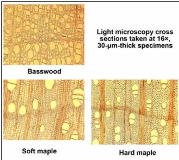
**Figure 10–4. Cross sections of three different species showing openness of cellular structure. Basswood is in the “bond easily” category in Table 10–1, soft maple “bond well,” and hard maple “bond satisfactorily.” The more easily bonded wood has greater lumen volume for adhesive penetration and less cell wall volume. The lower density of the basswood compared with the hard maple makes the wood weak, and therefore less force can be applied to the bondline.**
