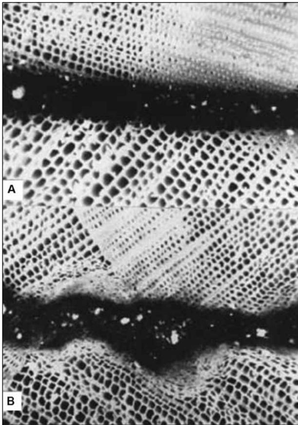
**Figure 10–2. Cross sections of bonded joints involving undamaged and damaged Douglas-fir surfaces. The dark area at the center of micrograph is the adhesive bondline. Image A involves two undamaged surfaces from planing with sharp knife (120×) and shows open wood cells with their distinct walls. Image B involves two damaged surfaces abrasively planed with 36-grit sandpaper and shows crushed cells with their indistinct walls in and adjacent to the bondline.**
