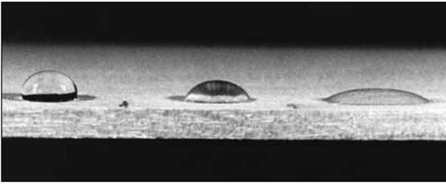
**Figure 10–3. A simple water drop test shows differences in wettability of yellow birch veneer surface. Three drops were applied to surface simultaneously and then photographed after 30 s. Left drop retained a large contact angle on aged and unsanded surface; center drop had a smaller contact angle and improved wettability after the surface was renewed by two passes with 320-grit sandpaper; right drop showed a small contact angle and good wettability after four passes with the sandpaper.**
