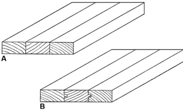
Figure 10-9. Edge-grain joints: A, plain; B, tongue-and-groove.
