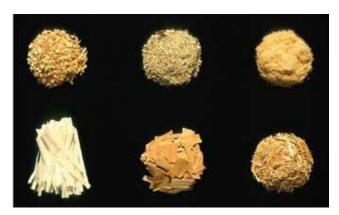
Figure 11–5. Common wood elements used in woodbased composites from top left, clockwise: shavings, sawdust, fiber, large particles, wafers, and strands.
