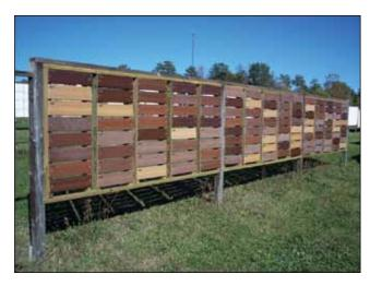
Figure 11–17. Extruded wood–thermoplastic composites being evaluated for a siding application (Clemons and Stark 2007).
