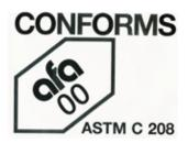
Figure 11–12. Typical grade stamp for cellulosic fiberboard. (Courtesy American Fiberboard Association, Palatine, Illinois. Used by permission.)
