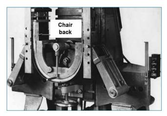
Figure 19–1. Chair back being bent through an arc of 180° in a bending machine.
