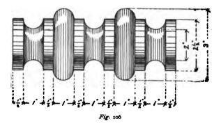
Turn a plain cylinder 3 inches in diameter, mark on it the lines that determine the convex curves, and reduce the remainder of the stock to a diameter of 2½ inches, and then cut the convex curves. Next, mark the position of the concave curves and cut them in the same manner that the concave curves were cut in the regular fourth exercise.
