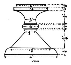
Put the second piece of stock between the lathe-centres, and turn from it the stem to the form and dimensions shown in Fig. 92. Varnish and polish it before taking it from the lathe.
