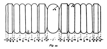
It will be found better to first cut grooves at the points of division, as shown in Fig. 45, as this helps to define the beads and keeps the size more nearly right. These grooves are cut in the same manner that the recesses in the second exercise were cut—with the acute corner of the chisel, the obtuse corner being held clear of the surface being cut. Use the obtuse corner in cutting the convex curves. Place
