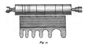
the parting-tool, cut grooves into the wood where the marks were made, using the notches cut from the edge of the templet, instead of the calipers, to de-
