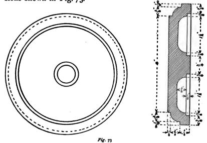
Fasten the disk to a face-plate with \(\frac{3}{4}\)-inch screws, placing the centre of the plate over the centre of the disk, and selecting such a face-plate that the holes left in the disk by the screws will be cut away in the subsequent turning—that is, the holes made by the screws must come in some place where a recess will be turned in the disk. Screw the face-plate easily on the spindle of the head-
