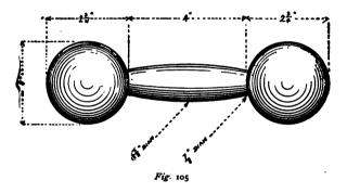
Next, find the centre of each of the larger parts, and mark it around with a pencil, and, using these centre lines as the starting-places for cuts, turn each end to the spherical form shown in Fig. 97, operating in the same manner that the convex curves were made in the regular third exercise. Turn the inside first and then the outside, cutting the ball a small amount inside the outer corner, that the spherical
