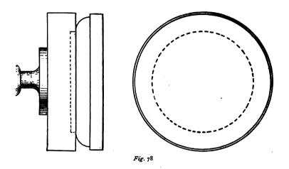
Next mark on the face of the outer disk a circle 4 inches in diameter and another  $\frac{3}{4}$  inch in diameter, and cut a recess  $\frac{1}{8}$  inch in depth between these marks with the skew
