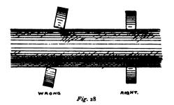
better to stop the lathe when using the calipers during the few first exercises, though, later, they may be used while the work is revolving.
