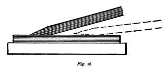
The edge left by the grindstone is too rough for use in turning, so to secure the necessary smoothness and to further sharpen the tool the whetstone is used. The chisel is applied to the whetstone with the same care with which it was applied to the grindstone. It is first placed in the position shown by the dotted lines in Fig. 16, then raised
