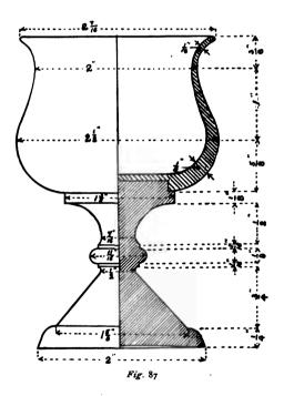
Prepare a chuck by attaching a piece of pine wood, four or five inches in diameter and one inch thick, to a face-plate, and turning it round and smooth: after which, with the face-plate still attached, remove it from the lathe and fasten to it the disk from which the bowl of the cup is This may to be made. be done by inserting a screw from the back through the opening for the lathe-spindle, as shown in Fig. 88.
