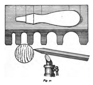
piece of sheet-iron, or of wood and iron, as shown in the sketch, or be entirely of wood. The principal dimensions for length are notched on one edge, and the caliper sizes to correspond are cut out of the other, as shown in Fig. 70.
