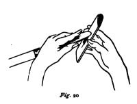
The round-nose tool is made from a narrow carpenter's chisel, and is ground and
