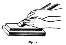
Fig. 17. The chisel is held in the right hand, and the fingers of the left hand used to steady it. When the sharpening is nearly complete, the tool is frequently turned over from one bevel to the other and given a few rubs on each. Any fine wire edge now formed may be removed,
