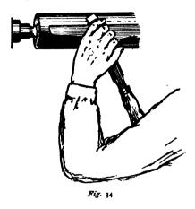
may be used as a guide in regulating the depth of the cut as the cutting edge is advanced to the end of the wood. Start the cut about 2 inches from the tail-stock end and produce it to the other end.
