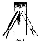
as before, by drawing the edge through a piece of wood, or it may be "buffed" off by rubbing the edge on a leather strap or on the palm of the left hand.
