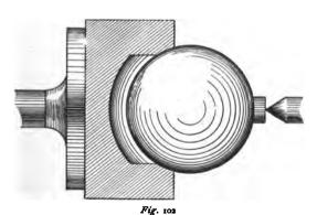
Prepare a chuck of the form shown in Fig. 102, and fit it to the ball, as shown. The ball may be held in place by putting a small piece of thick leather against
