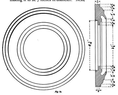
turn a recess in the face 4½ inches in diameter and § inch in depth, and when this is done remove it from the face-plate. Put on instead of the disk just turned a pine one
