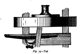
scraping inas stead of a cutting tool-turn the edge of the revolving disk true, making the diameter to be 5 inches. Next "face" the disk by holding the same chisel in the position shown by the views of Fig. 75, one corner of the chisel having contact with the work, and make the face flat and smooth by advancing the chisel across the work in the direction of the corner having contact. The chisel must be sharp, or the work will not be smooth.
