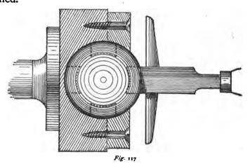
Over the wooden chuck used in turning the ball fit a wooden disk, and turn a hole in the centre of it, so that it may be fastened to the chuck with screws, and have a portion of
