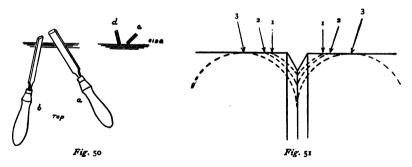
The aim should be to so combine the features shown that the cut will be a smooth and continuous one.
