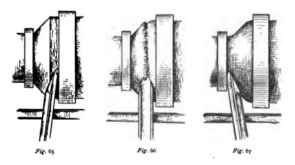
being used supported, by having the part of the bevel directly behind it in contact with the revolving stock, and the corresponding part of the back of the chisel in contact with the tee rest, as shown in the sketches. The gouge must be grasped quite firmly, and the handle raised slightly during the cut. The cut is started against the shoulder on the right-hand side and finished against the one on the left-hand side of the curve to be cut.
