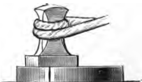
Fig. 89.—Smoothing Faces of Ring with Flatter.
