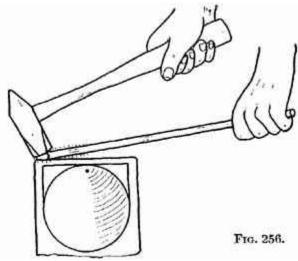
Fig. 256.--In pointing a rod d or bar, raise the back end, tilt the toe of the hammer down, and work on the far edge of the anvil. Round points should be made square first, then eight-sided, and finally round.
