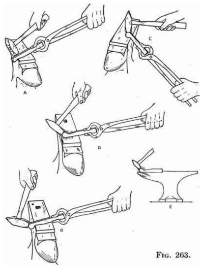
Fig. 263.-Forming a shoulder or neck, preparatory to punching a hole for an eye. The iron is first driven down against a corner of the anvil, as shown at (A). The end of the piece is then shaped and rounded by working over the corners and the horn of the anvil, as suggested in the various other views.
