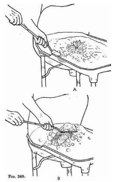
Fig. 249.-The forge fire should be cleaned by pushing the shovel along the bottom of the hearth to the center of the fire, as at A, and then lifting it straight up, as at B. The clinker and ashes, if any, will be exposed and can be easily removed.
