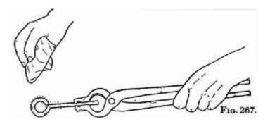
Fig. 267.-An iron may be blacked by heating it slightly and rubbing I ing it with an oily rag. The iron should be just hot enough to make the rag smoke. Blacking improves the appearance and affords some protection against rusting.
