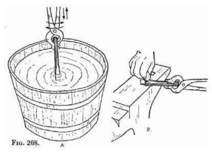
Fig. 268.-Tempering a cold chisel.
