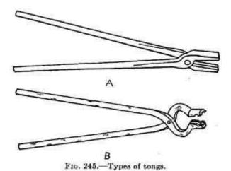
Fig. 245.-Types of tongs. (A). Flat-jawed hollow-bit tongs. (B). Hollow-bit curved-lip tongs. This style is very good for the farm shop. Flat bars as well as round rods and bolts can be held in them.
