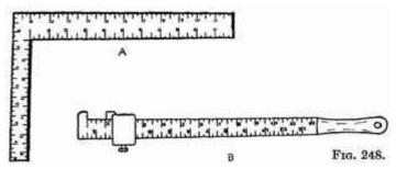
Fig. 248.-Metal measuring tools should be used in blacksmithing. (A). The small steel square is very useful for checking bends and angles as well as for measuring. (B). The caliper rule is especially good for measuring the diameter or thickness of bolts, rods, and bars; as well as for general measuring.
