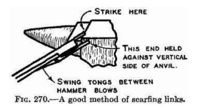
Fig. 270.-A good method of scarfing links.
