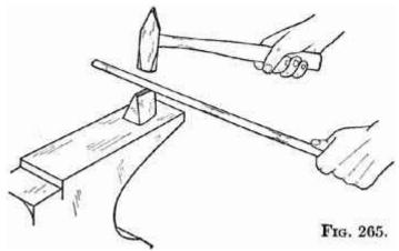
Fig. 265.-Iron may be cut either er hot or cold on the hardy. Cold iron may be nicked deeply on two or three sides and broken by bending. In cutting hot iron, cut all the way through from one side, being careful to strike overhanging blows at the last to prevent the hammer from striking the cutting edge.
