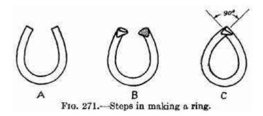
Fig. 271-Steps in making a ring.
