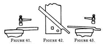
Third—Form second step. Turn the work to the left and form shoulder even with the first, on the sharp edge of the anvil. Hold at about  $60^{\circ}$  as shown in Figure 42.
