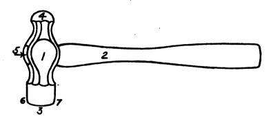
FIGURE 3. NAMES OF PARTS OF HAMMER.
