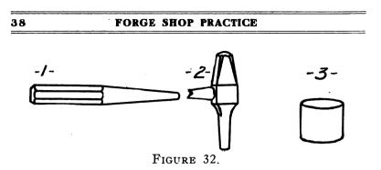
Fourth—Punch the hole in center of the eye, using blacksmith punch. (1—Figure 32.) (Note. After starting the punch, remove it to see if the hole is in the center of the eye. If not, change it; drive the punch about half way through; turn work over and repeat the process on the other side; place the work over the round hole in the anvil and drive out the burr.
