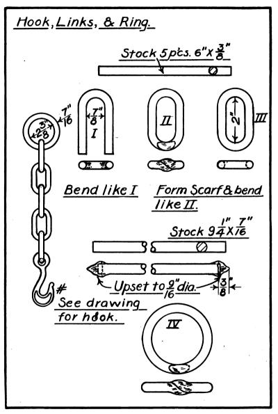
*Third*—Scarf and bend, ready for welding like II. Figure 25 shows the proper position for scarfing.
