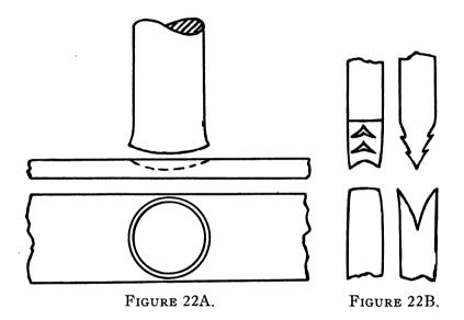
The Cleft or Fork Weld. A weld of this sort is used for heavy stock. One piece is split in the shape of a Y and the other is tapered to a blunt point. This weld is used in joining iron to steel, being closed together before heated for welding. Separate heats cannot be taken in welding tool steel. (Figure 22B.) Minor welds are "Angle" and "T" welds, the "angle" weld for flat stock and the "T" weld for flat or round stock.
