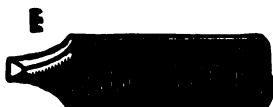
Fig. 368—Showing how the Forging is done at G, on the Other Piece.
