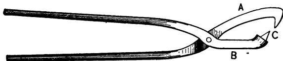
42—Iron Tongs for holding Bolt Heads, as made by E. K. Wehry.
