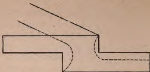
Fig. 134—Showing the Piece as Forged and Fullered.
