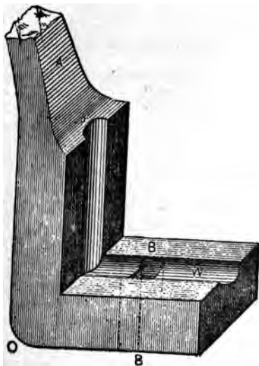
Making Shifting Rail Prop Irons. Fig. 219—Showing the Tool used to give the Iron a Complete Finish.
