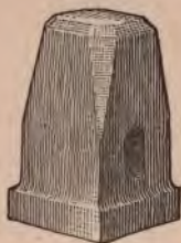
Fig. 5—Heavy Flatter for Straightening Cold Iron. Made of 2-inch square Steel.
