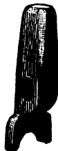
Fig. 2—Collaring Tool for Shouldering Down Round Iron. Made of 1\frac{1}{2} square Steel.
