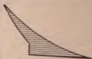
Fig. 363—Showing Piece of Iron as Used by "J. W. J." in Fitting Plowshare.
