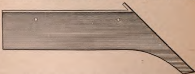
Fig. 342—Showing the Share Completed.
