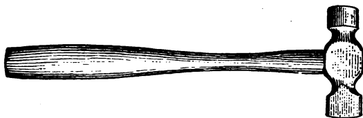
Fig. 345—Hammer Used by "J. W." in Welding Plow Points.
