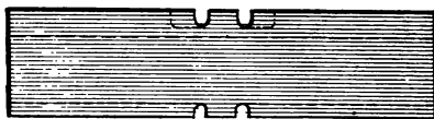
Fig. 195—Showing how the Fuller is used in making a Brewster Saddle Clip.
