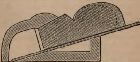
Fig. 8.—Bull-nose Plane in Section.
