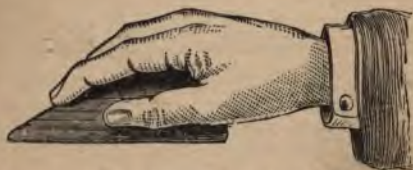
Fig. 6.—Method of holding the Rubber when in use.
