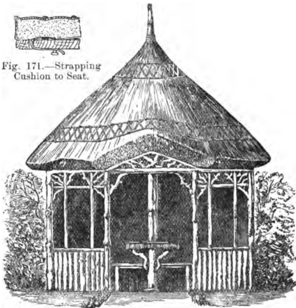
Fig. 172.—Front Elevation of Octagonal Summer-house.
