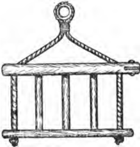
Fig. 109.—End View of Fenced Seat for Canopy.
