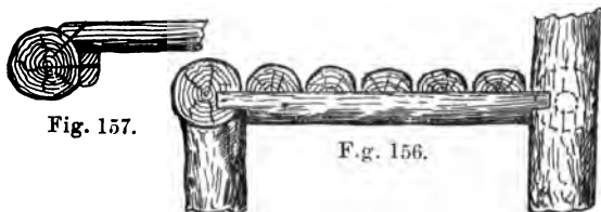
Fig. 156.—Section of Middle Rail at A (Fig. 152). Fig. 157.—Detail of Middle Rail at B (Fig. 152).
