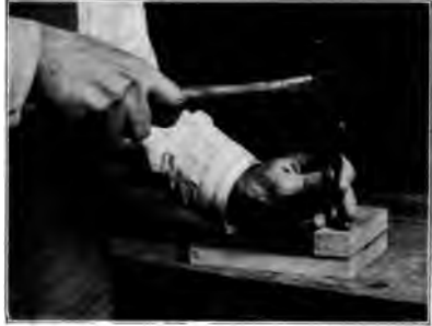
Fig. 165. Using a Nailset
