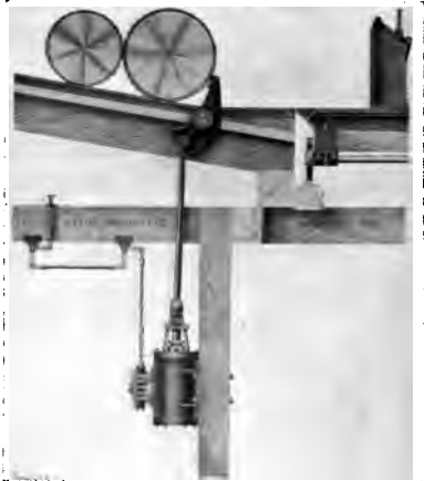
Fig. 39. Log-Stop and Loader. By letting steam into the cylinder, the projecting arm revolves, rolling one log over onto the carriage and holding the next one till wanted.
