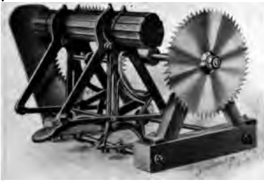
Fig. 51. Combination Lath-Binder and T-trimmer. With this machine the operator can trim the bundles of lath, simply by tilting the packing frame over from him causing the bundles to pass between the saws, thereby trimming both ends at one movement.
