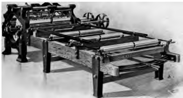
Fig. 43. Double Gang Edger. This machine trims off the rough edges of the "waney" boards by means of the four saws in the main frame of the machine.
