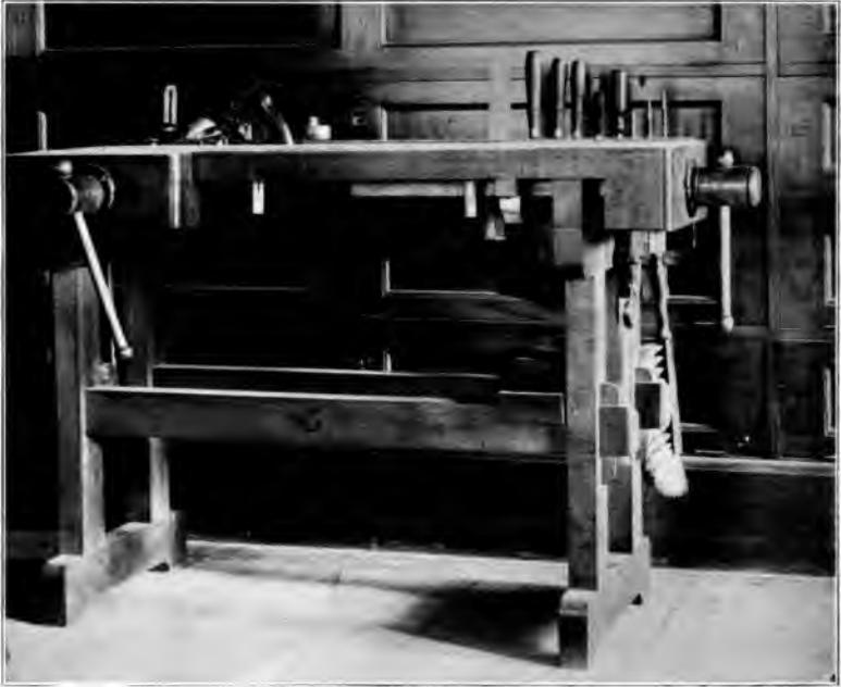
Fig. 166. Bench Made with Pinned Mortise-and-Tenon Joints, Low Back.
