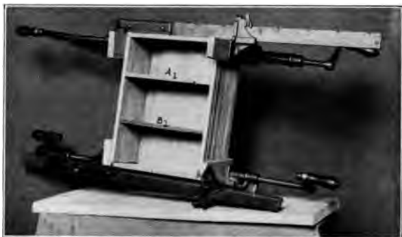
Fig. 286. Gluing Together a Box.
