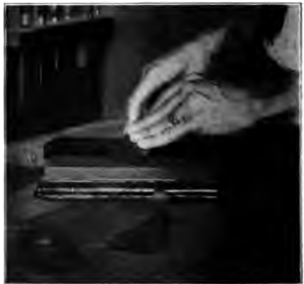
Fig. 77. Whetting a Plane-Bit.
