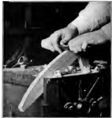
Fig. 120. Using a Spokeshave.
