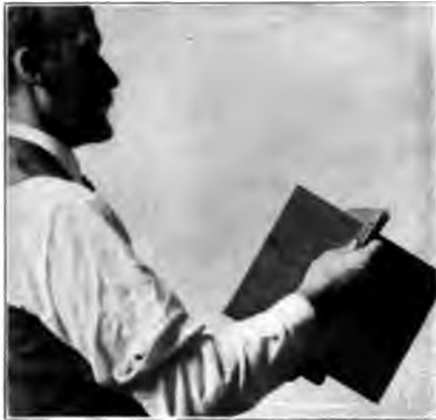
Fig. 203. Using the Try-Square.
