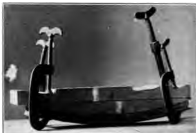
Fig. 299. Bending Boards into Shape after Boiling Them.
