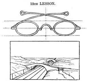
Vanishing points, for lines parallel to each other, and running away from spectator on a horizontal plane.
